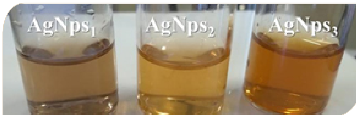
Figure 5. AgNps 1 , AgNps 2 y AgNps 3 samples with 0.5, 1, and 2 mL of the reducing agent, respectively
